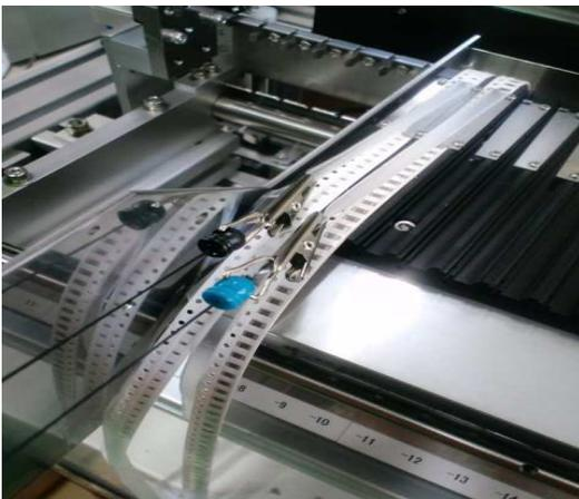
This case the cover tape is peeled off at the end of metal plate as usual auto tapes and edge of cover tape is clipped by rewind reel so the cover tape is gradually peeled off by advancing tape.
