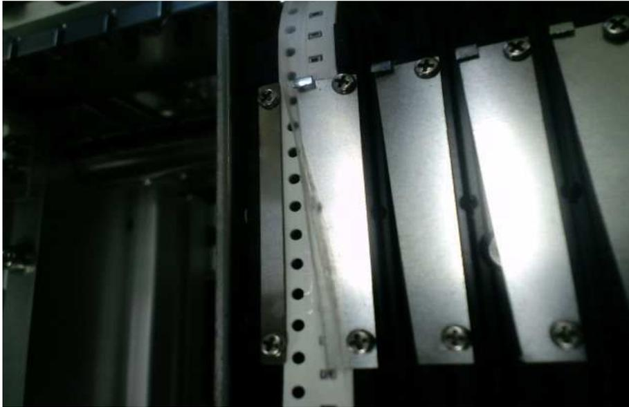
Loosen screws to insert tape since when shipping screws may be tighten. The auto cut tape system intends to peel off cover tape automatically by advancing action but some time it flips up chips and may not work with wider width components so other way to peel off cover tape is prepared as below.
