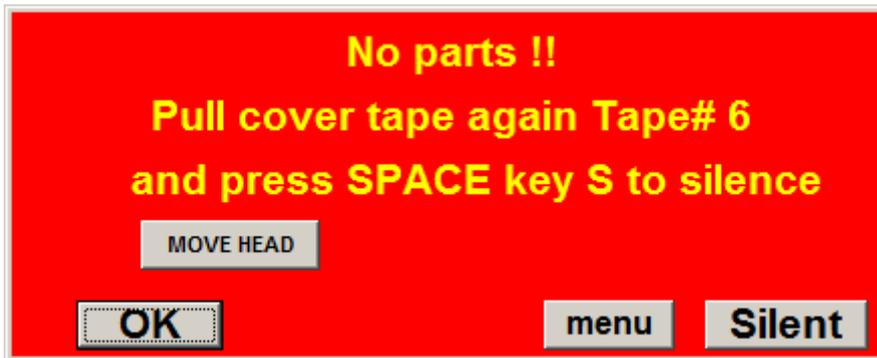
During assembly when numbers of picked up components reaches to qy then above warning is displayed so extend reel wire and clip the cover tape.
