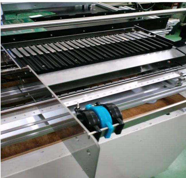
**This long prekit base occupies 20 auto tape slots and can set 5 8mm blocks (25 lane) or 4 8mm (20 lane) and one 12mm block (4 lane) etc. Short prekit base is also prepared for small block usage.**
