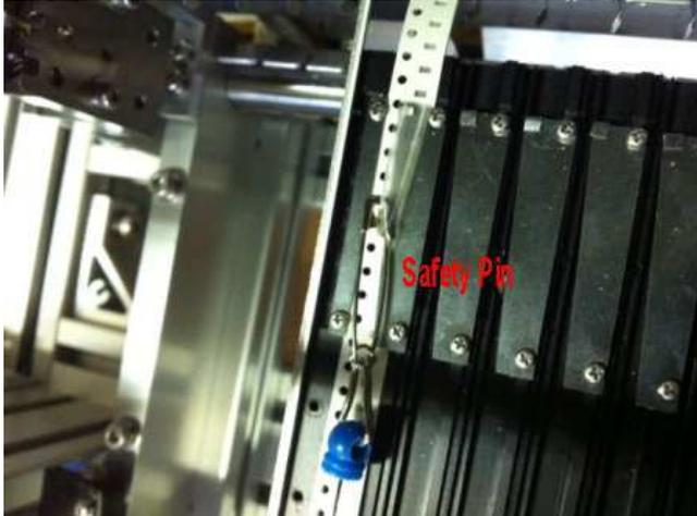
Modified safety pin is used for new shipment instead of alligator clip to avoid interfere with actuator.
