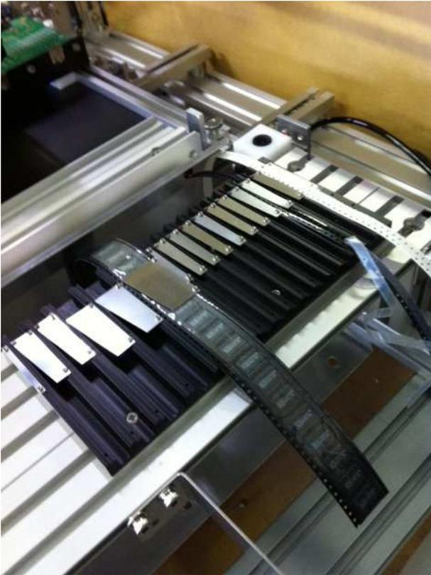
Full flat auto cut tape base is prepared for 7712 or 7702 model. It occupies full tape space on front or rear and can install 5 8mm blocks and 1 12mm block or other combined block.
