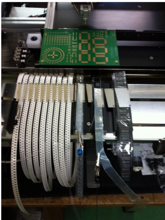
Cut tape blocks consist of 8mmx5, 12mmx4 and 12mmx2+16mmx2+24mm etc. and customer can choose them as required.
