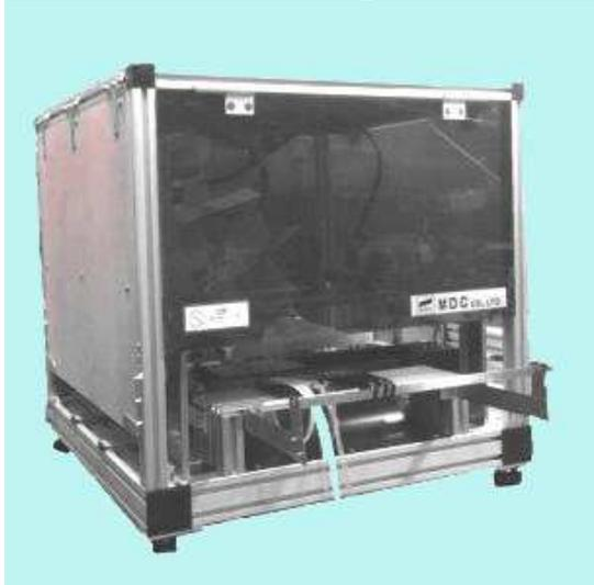
Handy full automatic pick & placer. It assumes approx 1000 chips per day production so it is suitable for prototyping and bread board assembly. PPP III model is larger than PPPII model slightly so it can hold larger PCB and rear side cut tape holder as option. PPP III model includes built in Vac pump so just mains power is necessary so easily set up any places just next to designer's desk.
